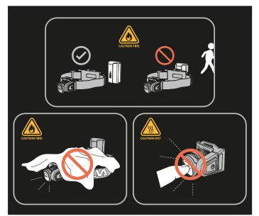
Note! Do not leave connected when unattended. Note! Do not cover or place in a pocket/toolbox while connected - risk of fire. Note! Be careful when handling the lamp unit with bare hands since it gets very hot. Do not touch the lens
